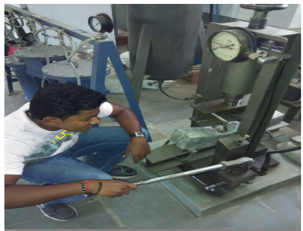
Figure-4 flexural strength testing set up.
