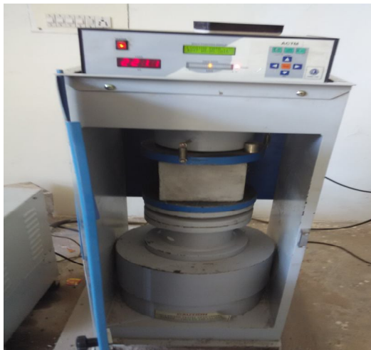
Figure-2 compressive strength testing machine
