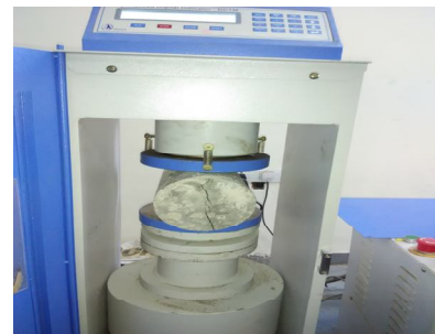
Figure-3 split tensile strength testing.
